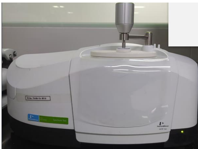
Figure 2. 11: Fourier transform infrared (FT-IR) spectroscopy, Perkin Elmer
