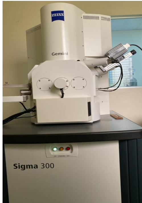
Figure 2. 12: Field Emission Scanning Electron Microscopy (FESEM), Model- Sigma 300 by Carl Zeiss AG, Germany
