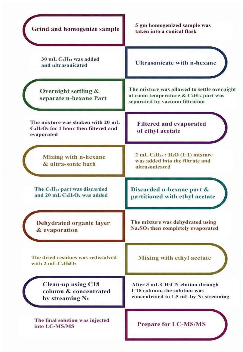
Scheme 5: Extraction and clean-up for antibiotic residues analysis in poultry feed samples
